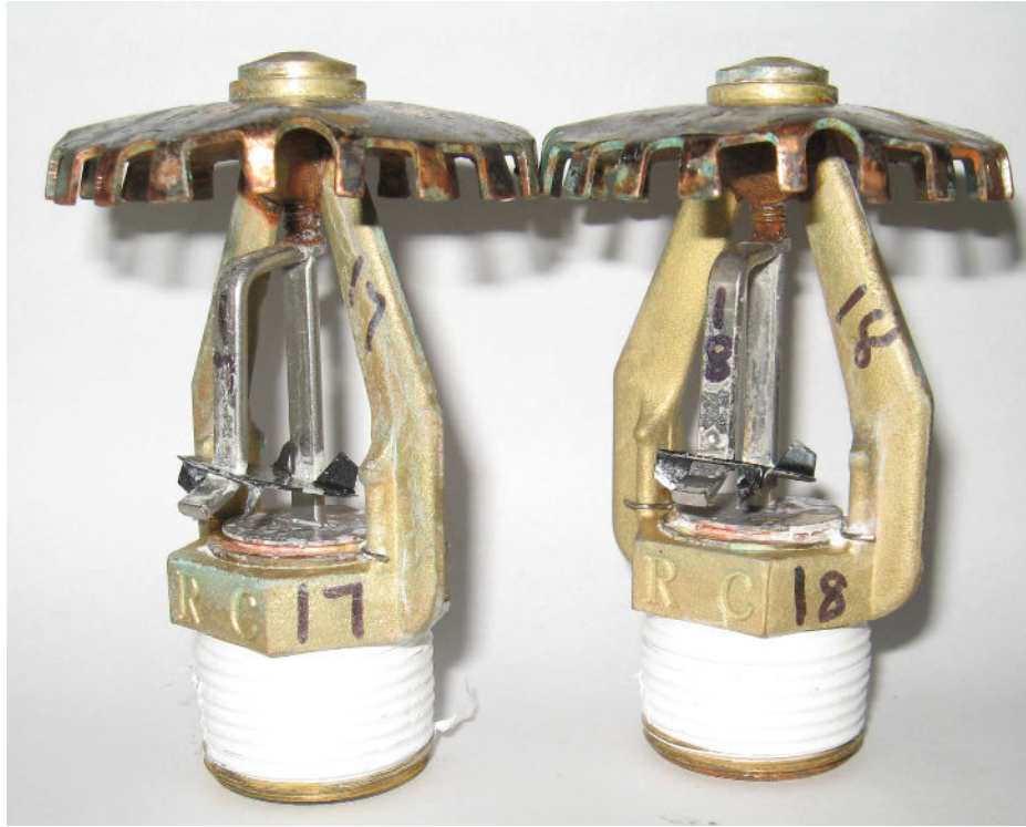
Figure 13 ESFR-363 10-Day Corrosion Samples, Post-Sensitivity Test
