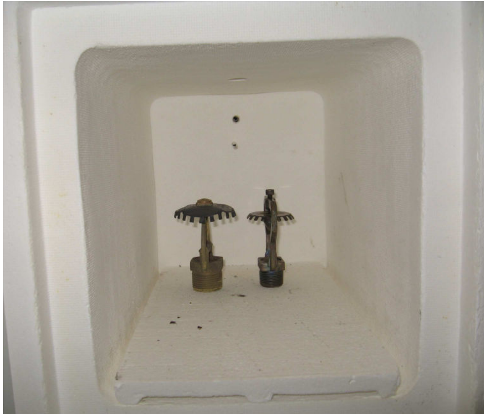
Figure 10 Heat Resistance Samples – Test Set-Up
