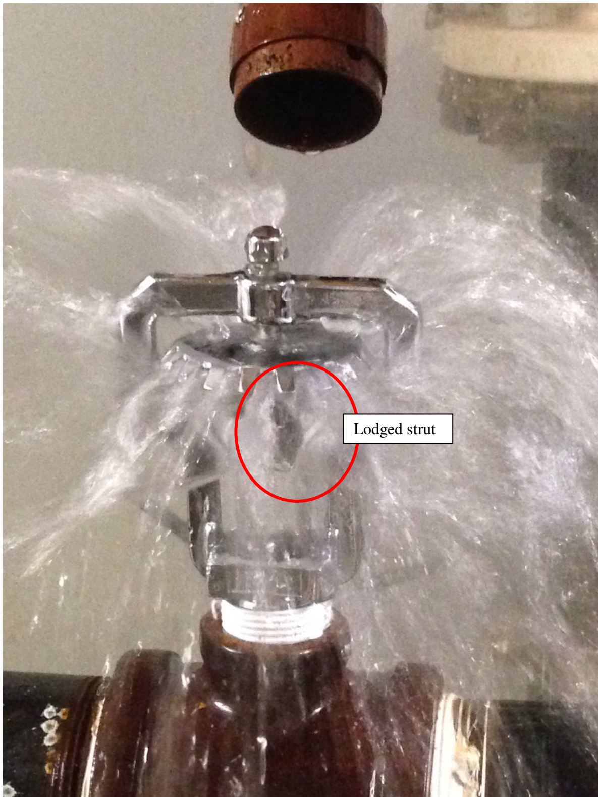
Figure 8 ESFR-202, Non-compliant Lodgment Test
