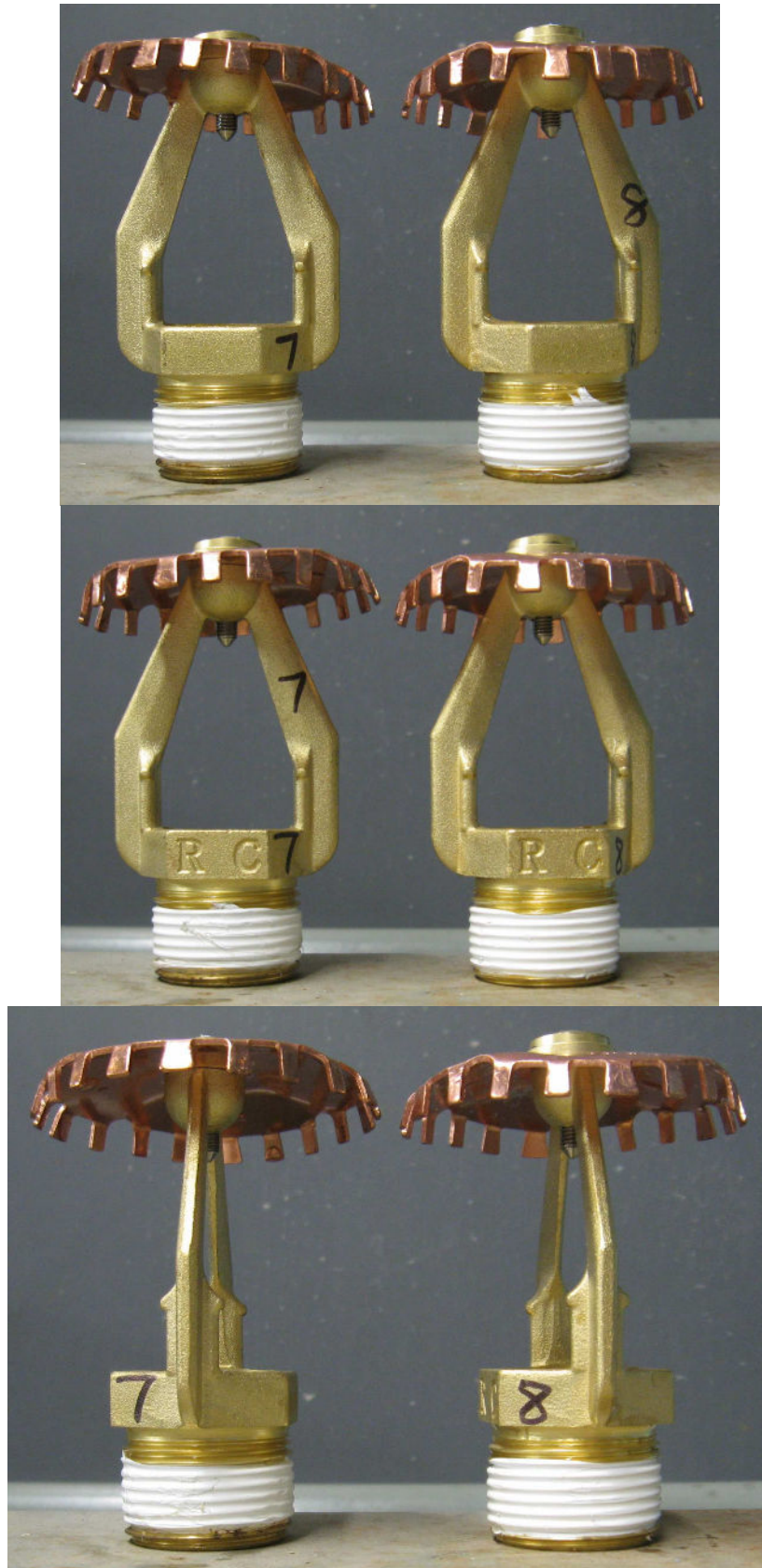
Figure 6 ESFR-363, Post-Flow Endurance Test – Deflector Deformation
